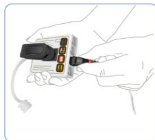
4. Connect Electrodes to Connection Cable & Box Match colored rings to color coded sockets
