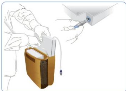
5. Place Device and Battery in Bag (if applicable) and Connect Battery or Power Supply
